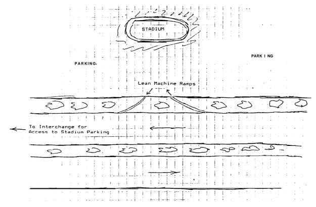
Figure 5. East-West Freeway Adjacent to a Stadium. Lean Machine on and off ramps provide additional capacity for eastbound entrance to parking and eastbound egress. Such ramps might be provided by adjoining property owners.
