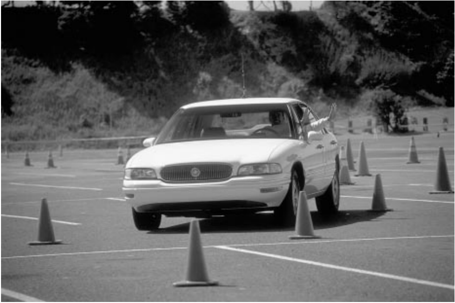
Figure 2.1 “Look, Ma, No Hands.” A demonstration of automated steering during the demonstration program of the NAHSC (Gerald Stone, California PATH Publications).
